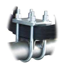
Tighten U-Bolts in the order shown. Torque to spec completely in the order shown. Check U-Bolts for tightness after 100 miles
